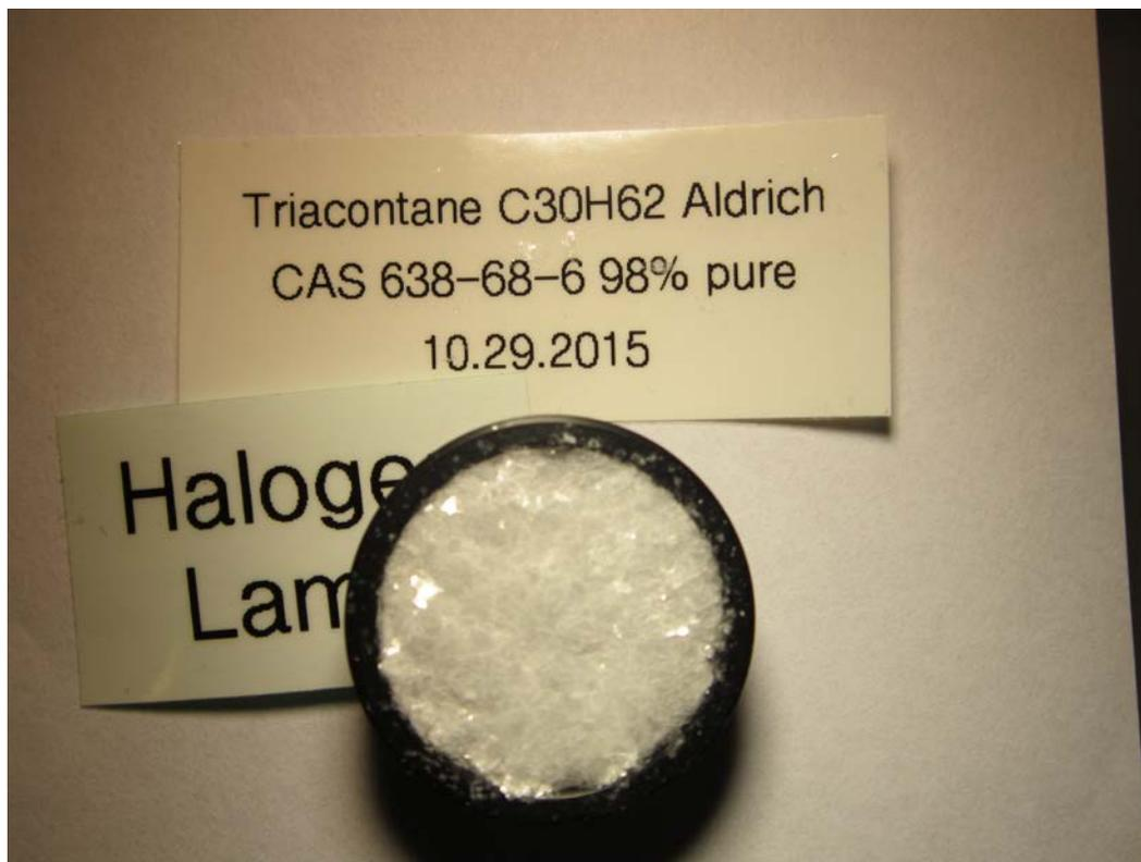
Figure 3: Triacontane loaded into IR sample cell.
