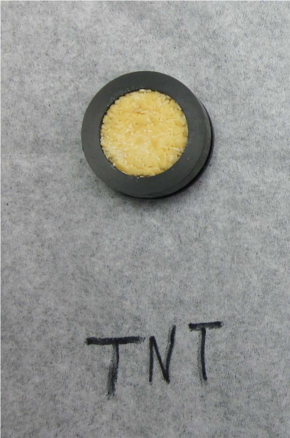
Figure 2: TNT in IR sample cup with a volume of 1.25 cm<sup>3</sup>.
