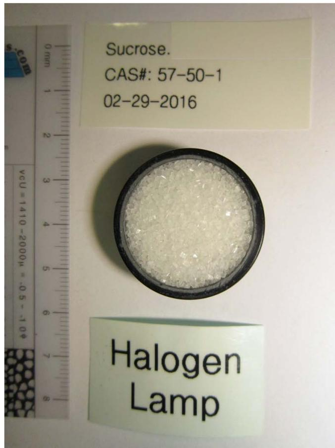
Figure 3: Sucrose sample loaded in IR sample cup.
