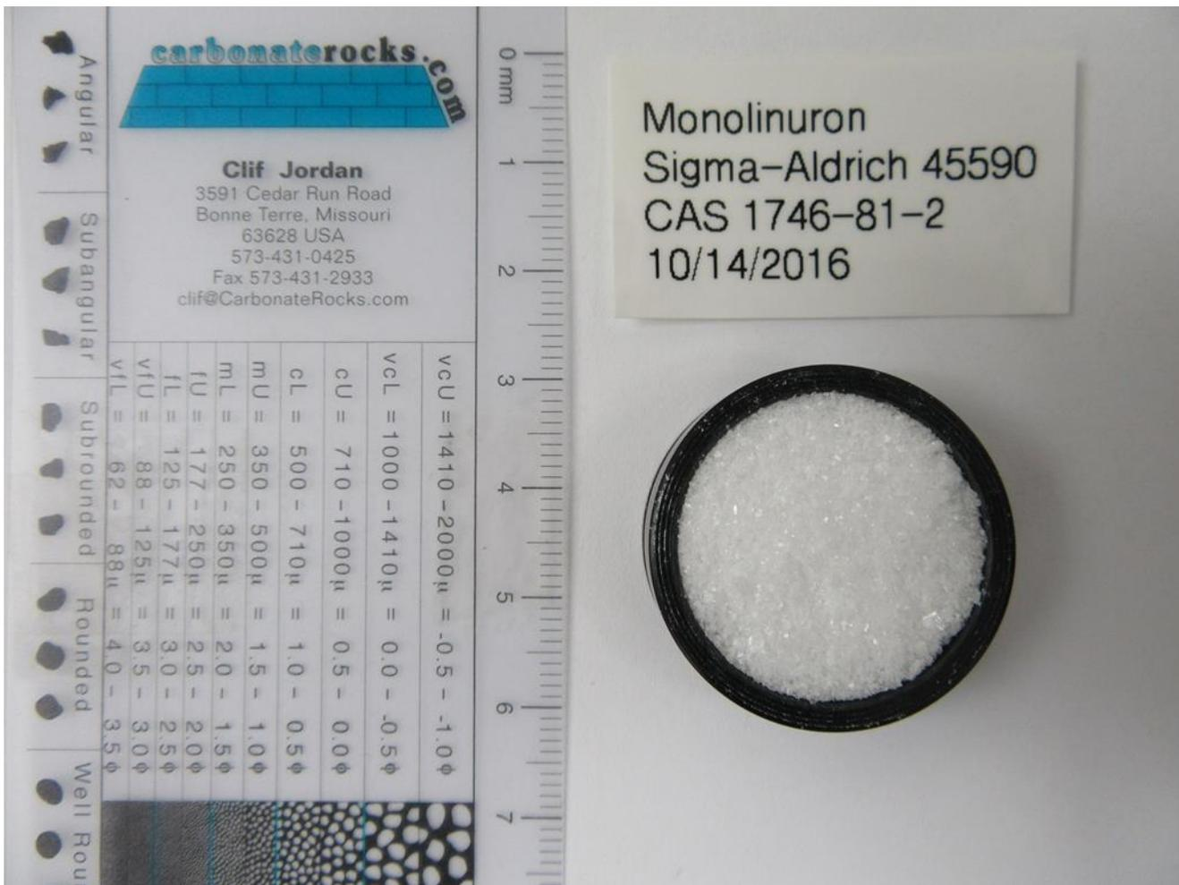
Figure 3: Monolinuron loaded in IR sample cup.
