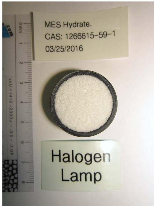
Figure 3: MES Hydrate loaded in IR sample cup.
