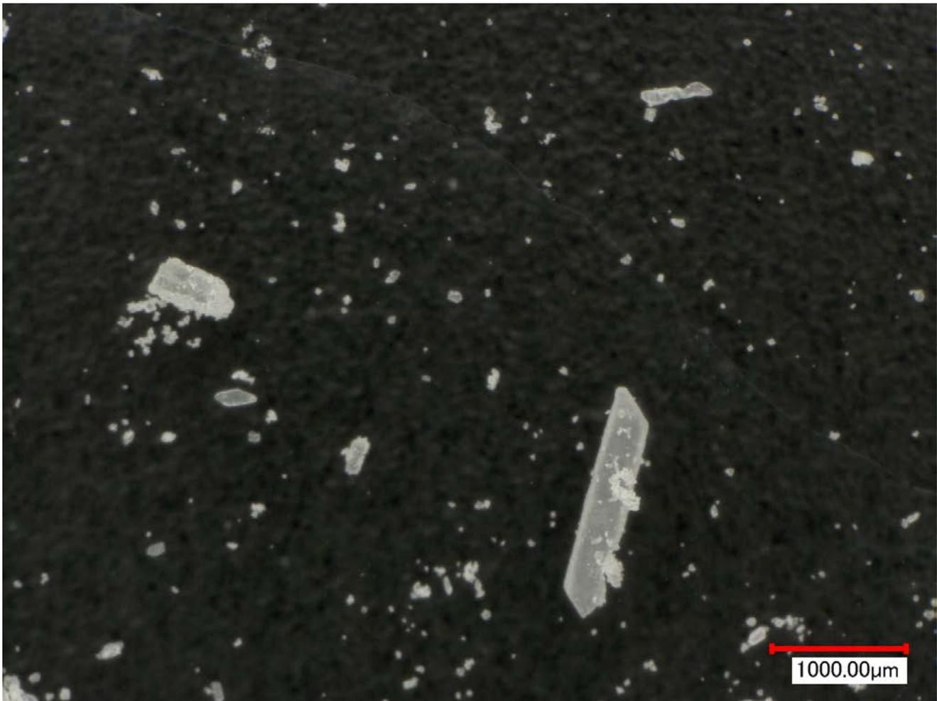
Figure 4: Photomicrograph of MES Hydrate.
