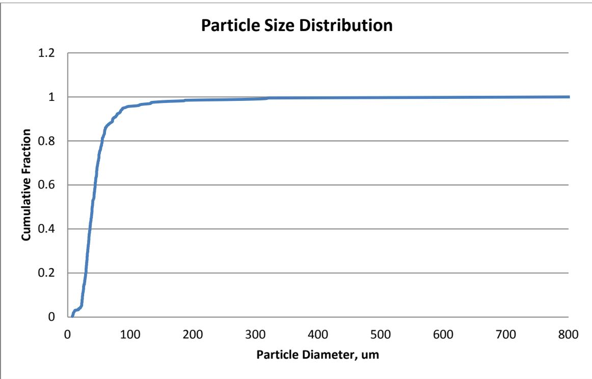
Figure 5: Particle size distribution of MES Hydrate.
