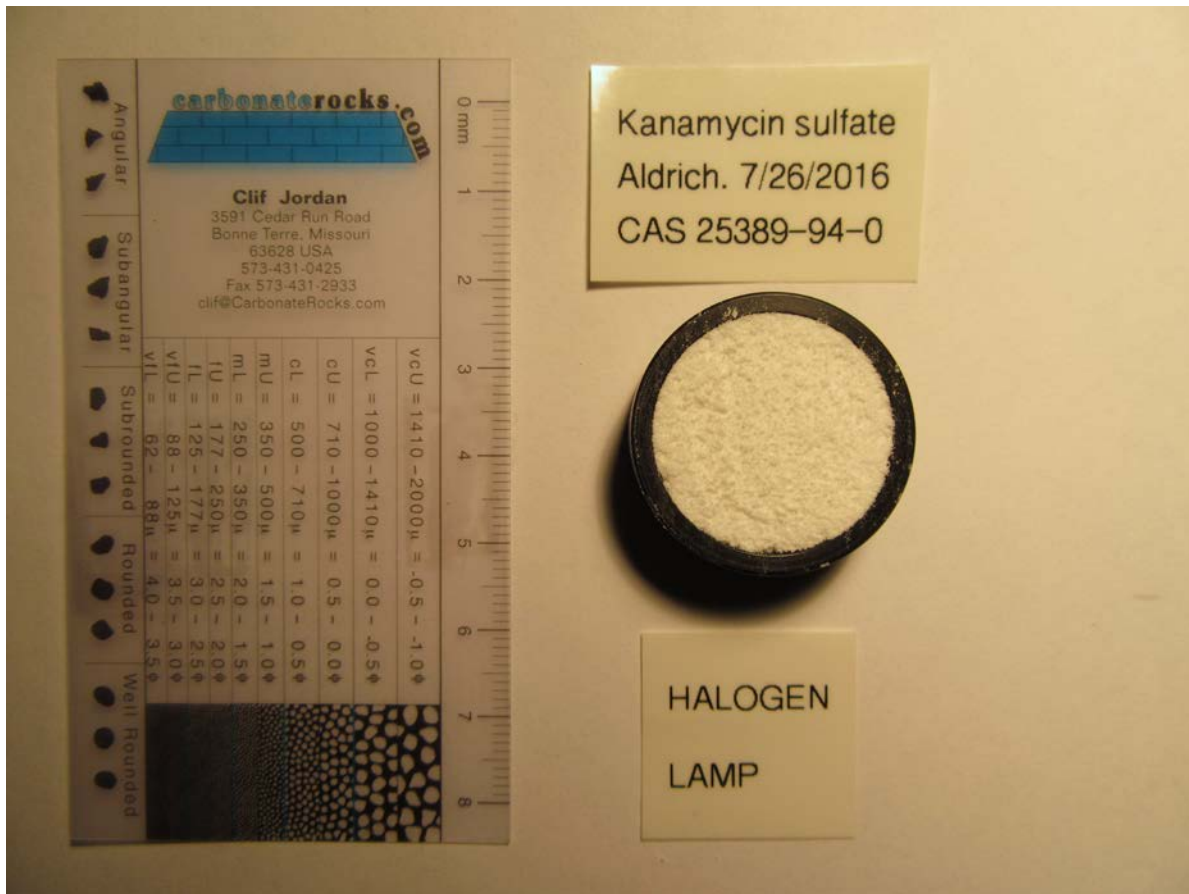
Figure 4: Kanamycin sulfate in IR sample cup
