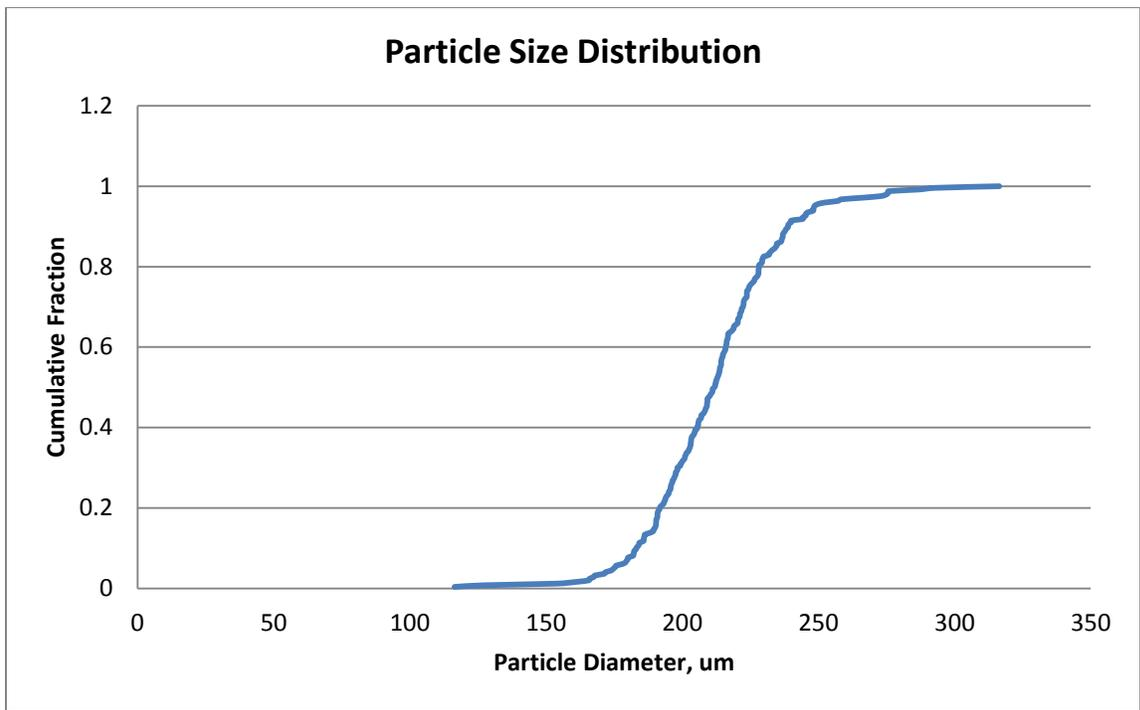
Figure 5: Particle size distribution of Glass Beads.
