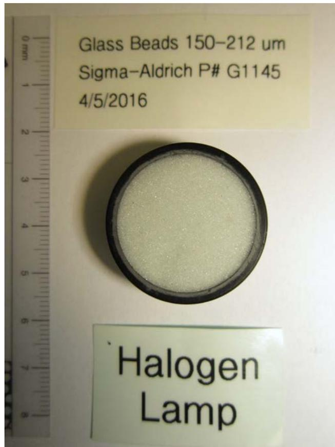
Figure 3: Glass Beads loaded in IR sample cup.
