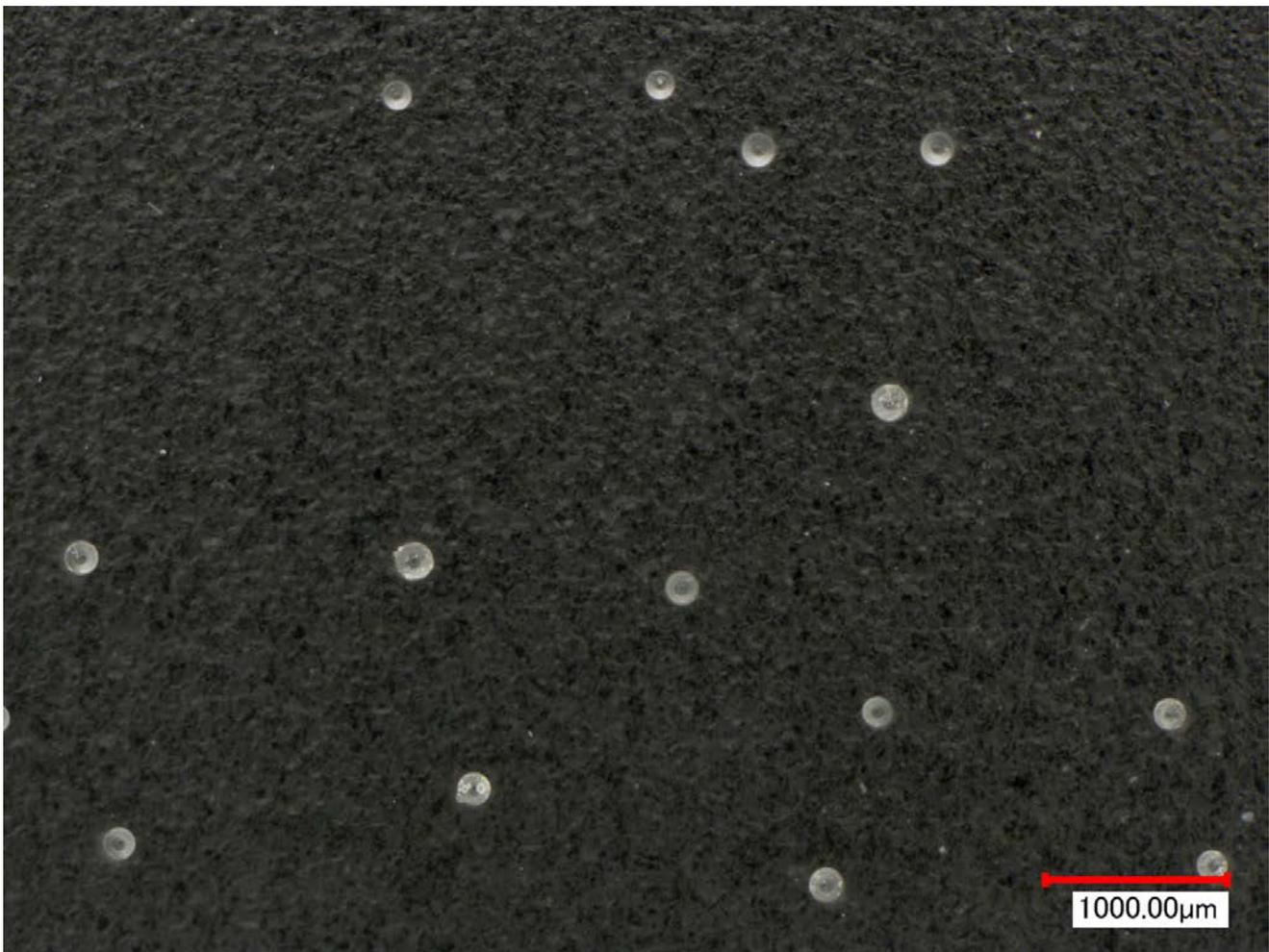
Figure 4: Photomicrograph of Glass Beads.
