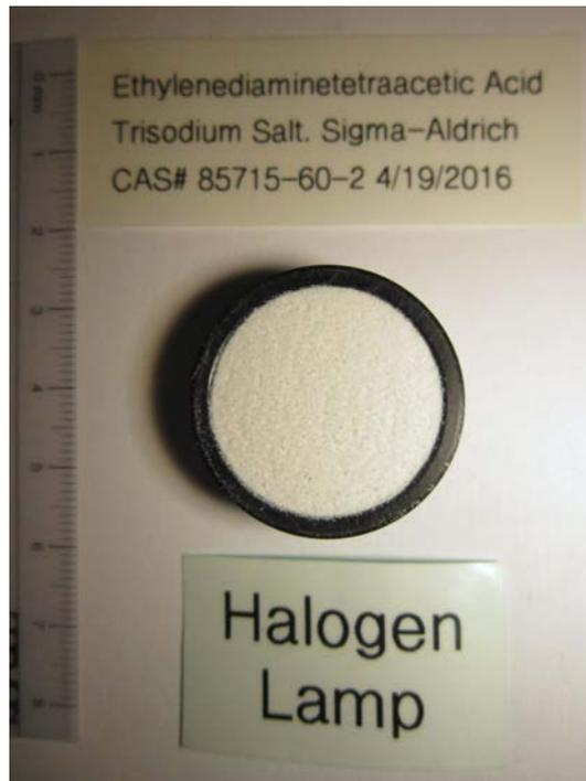
Figure 3: Ethylenediaminetetraacetic Acid Trisodium Salt loaded in IR sample cup.
