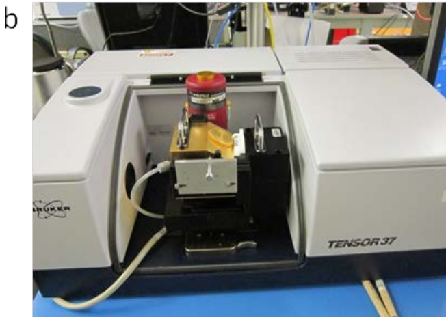
Figure 1: The Bruker 562-G integrating sphere (a) and Tensor 37 (b)
