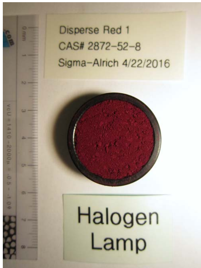
Figure 3: Disperse Red 1 loaded in IR sample cup.
