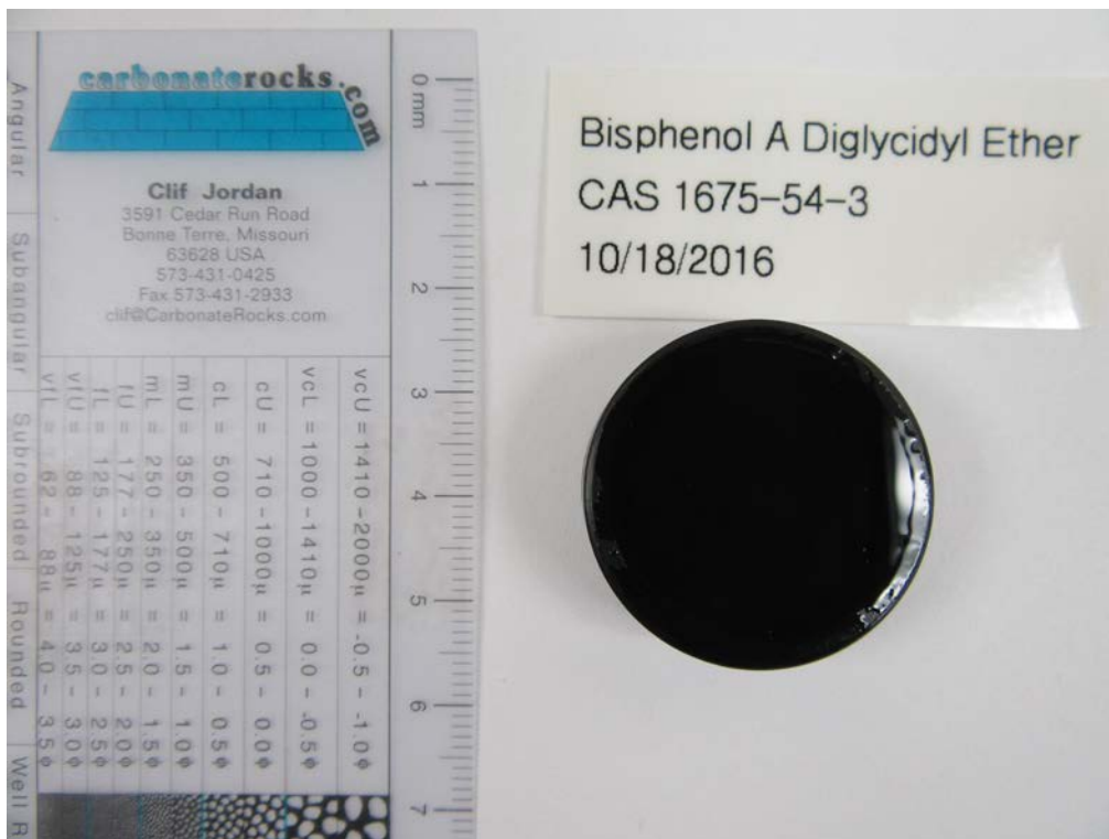
Figure 3: Bisphenol A diglycidyl ether loaded in IR sample cup.
