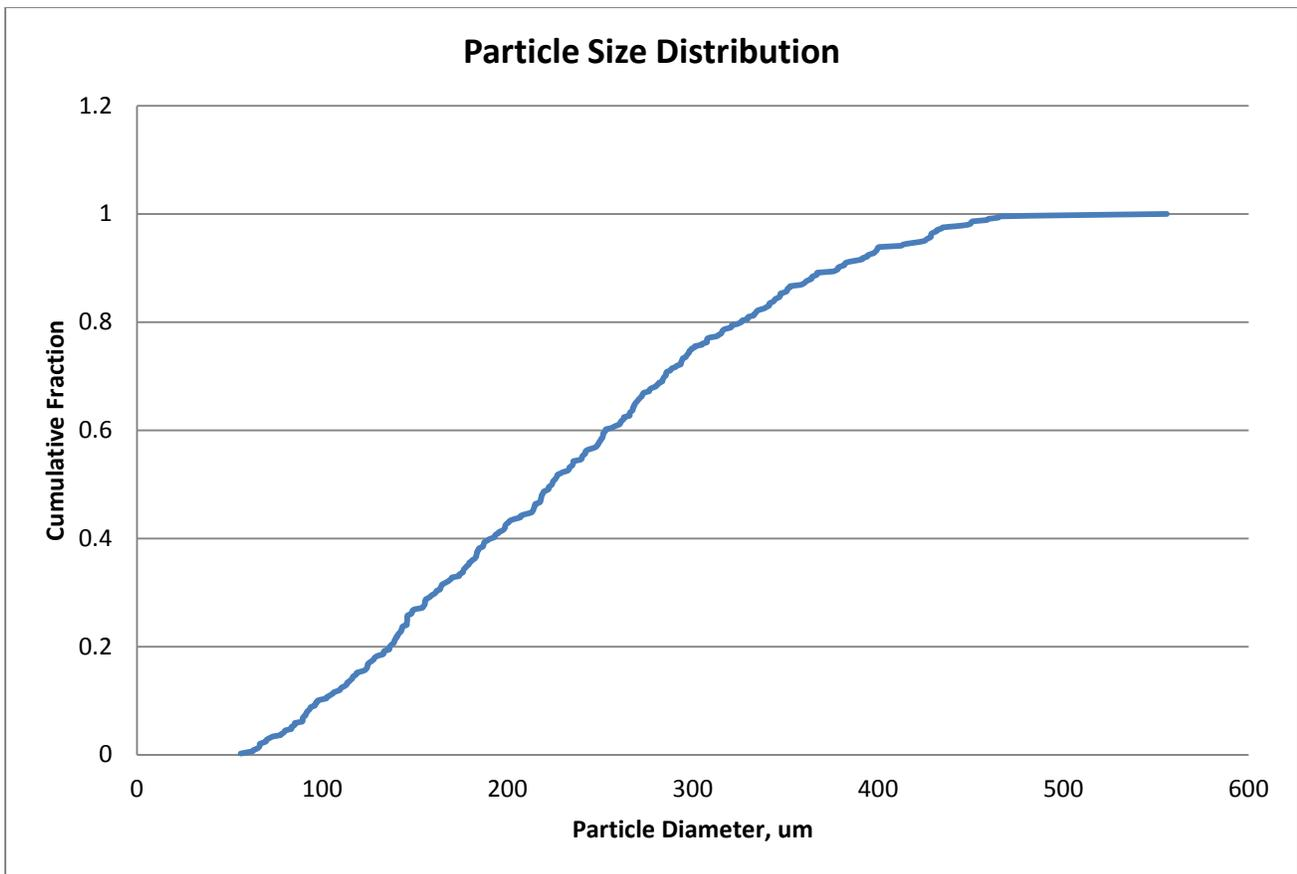
Figure 5: Particle size distribution of Ammonium perchlorate crystals.
