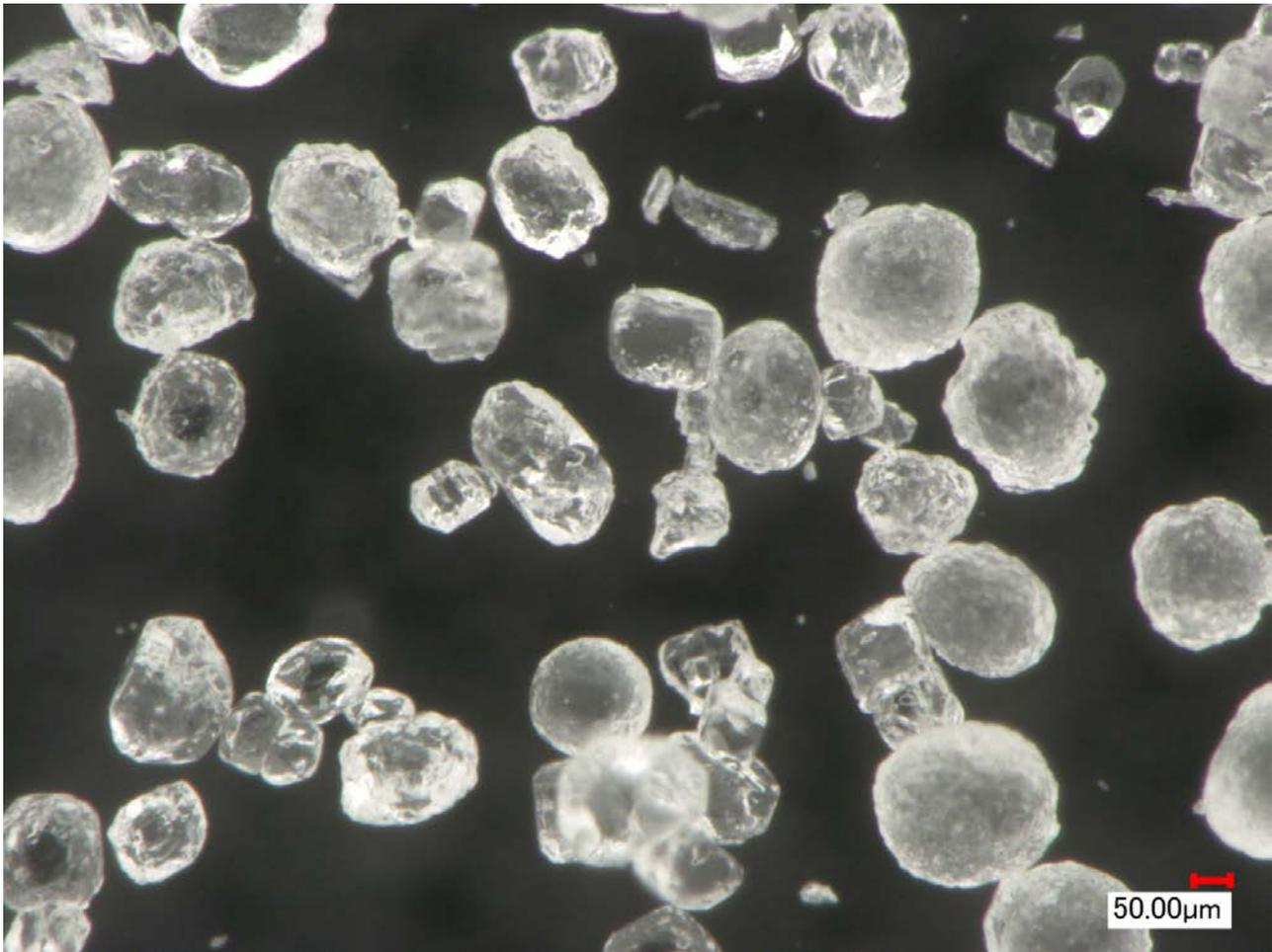
Figure 4: Photomicrograph of Ammonium perchlorate crystals.
