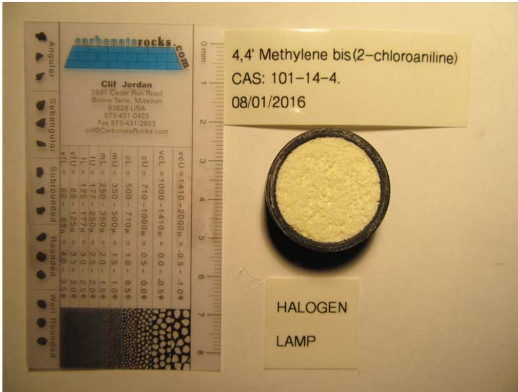
Figure 4: 4,4'-Methylene-bis(2-chloroaniline) ground in IR sample cup.
