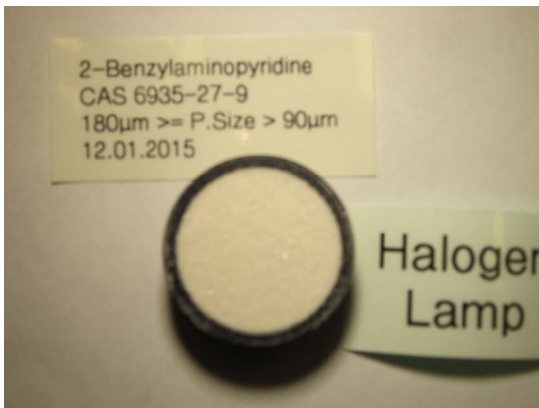
Figure 3: 2-Benzylaminopyridine 90-180 \mu\text{m} sample loaded in IR sample cup.
