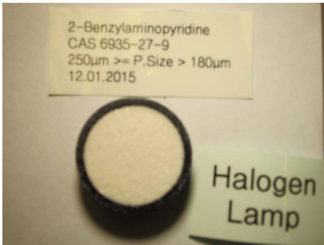
Figure 3: 2-Benzylaminopyridine 180-250  $\mu\text{m}$  sample loaded in IR sample cup.
