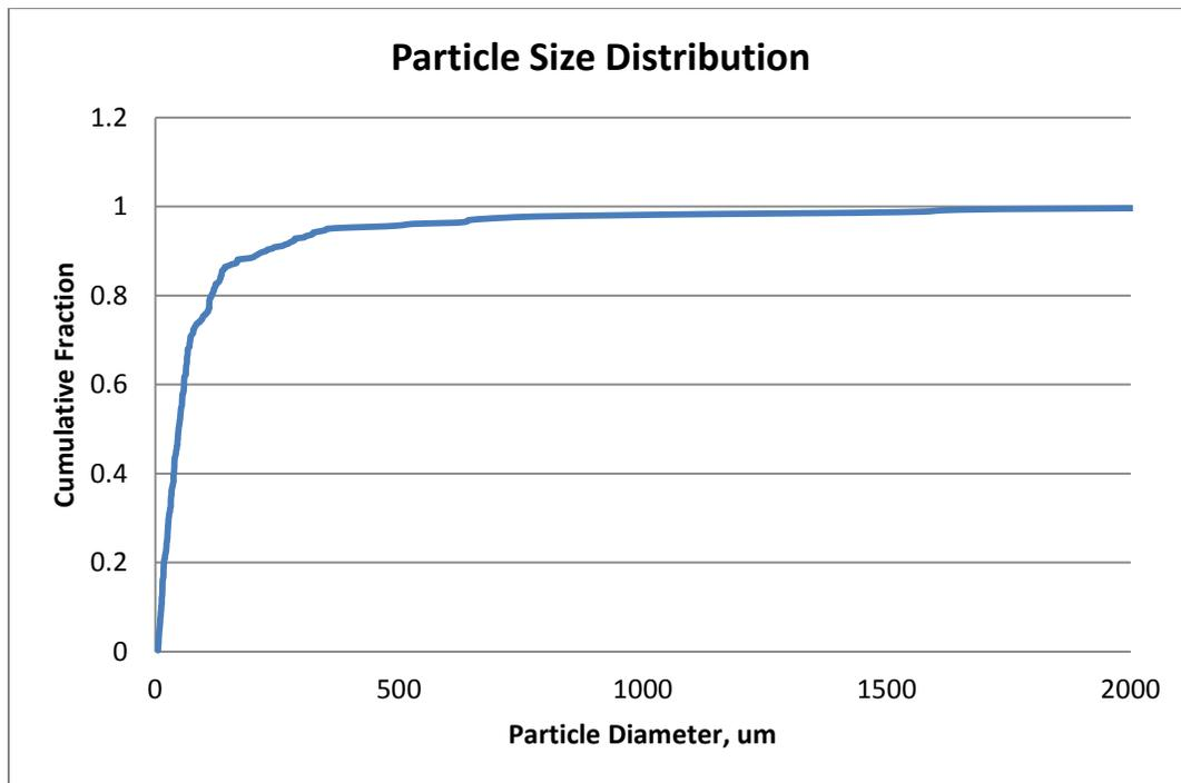
Figure 5: Particle size distribution of 2-(Dimethylamino)ethanethiol hydrochloride.
