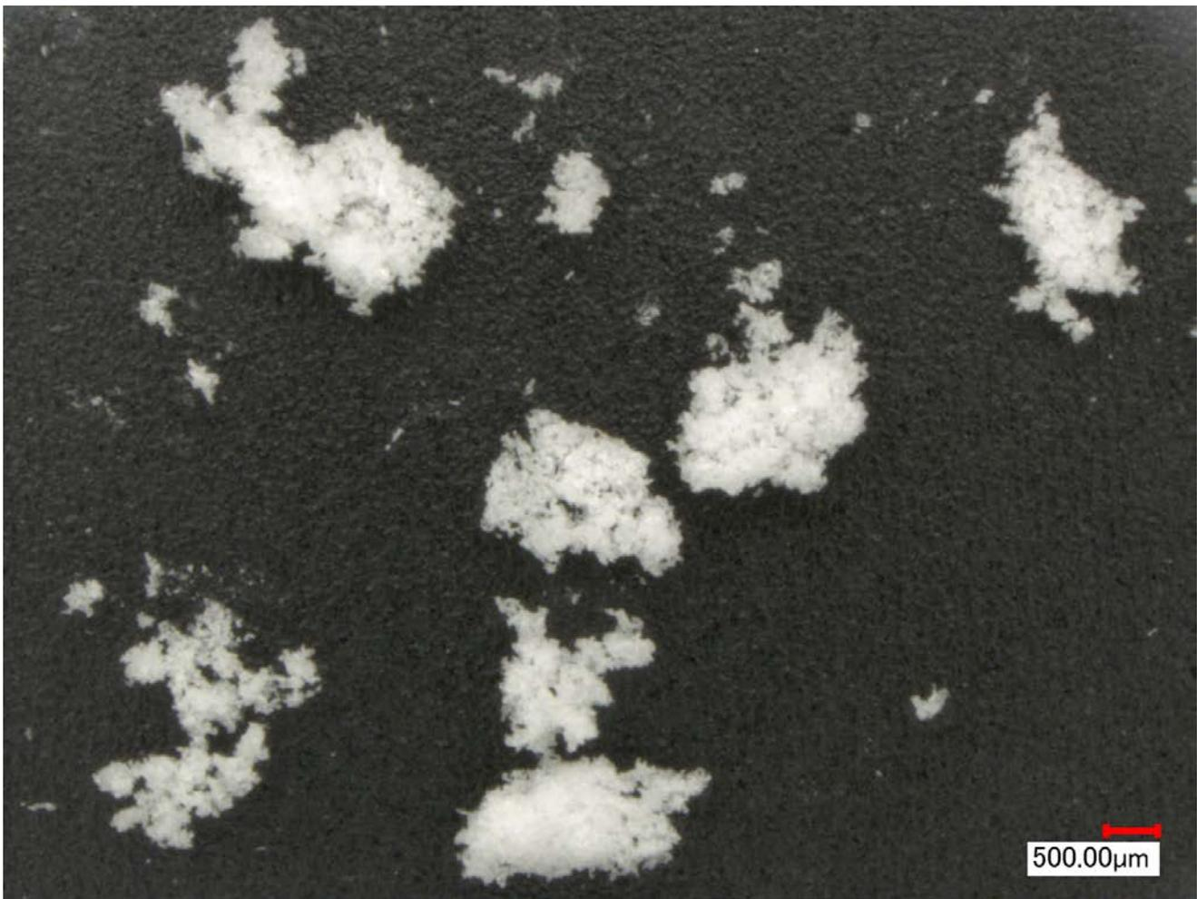
Figure 4: Photomicrograph of 2-(Dimethylamino)ethanethiol hydrochloride.
