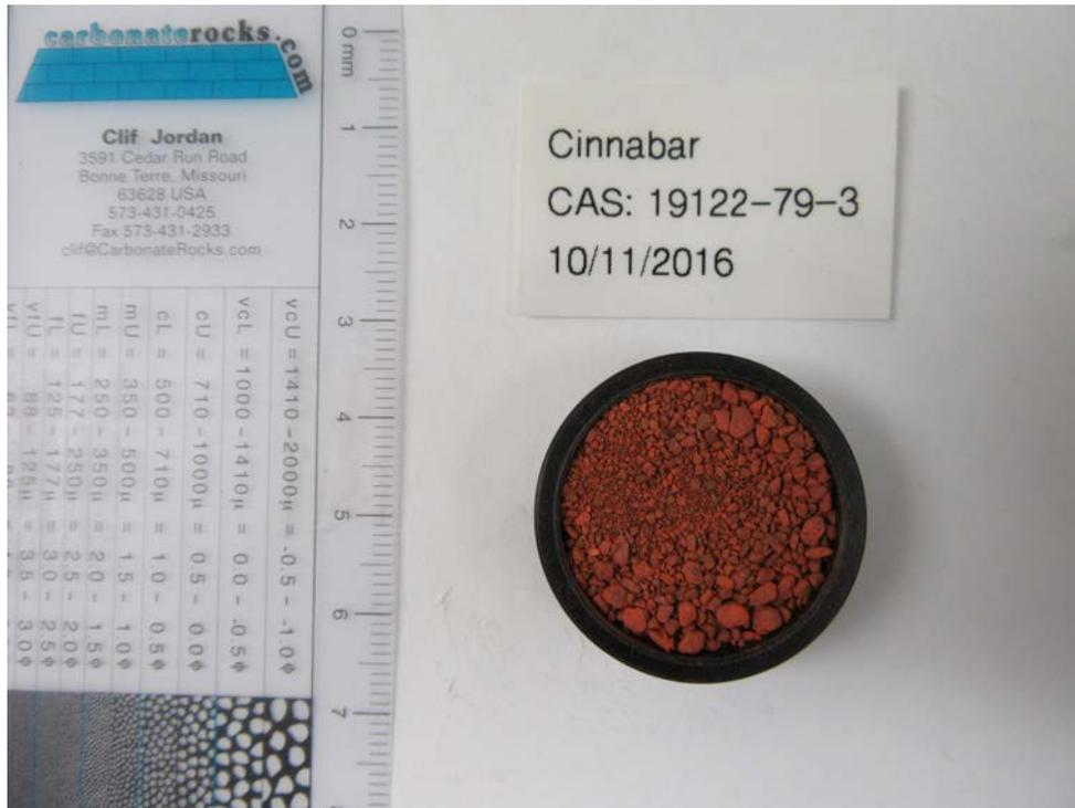
Figure 3: Cinnabar loaded in IR sample cup.
