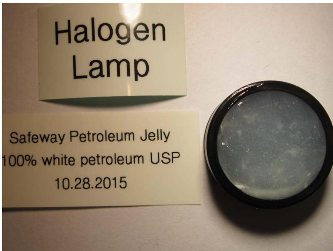
Figure 4: Petroleum Jelly loaded in IR sample cup.
