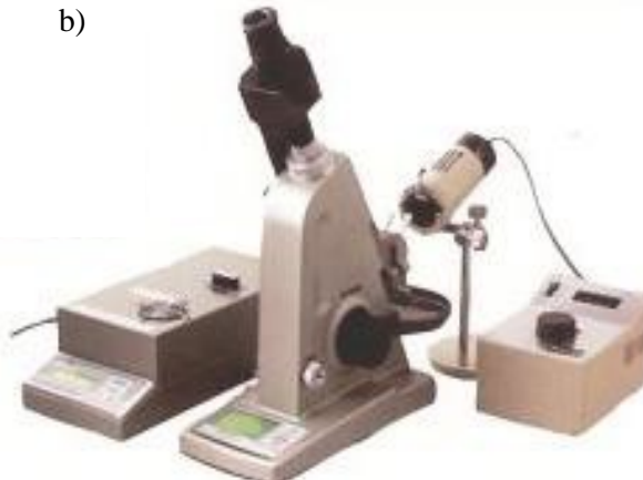
Figure 1: The Bruker Tensor 37 FTIR with HATR accessory (a) and Abbe refractometer (b).
